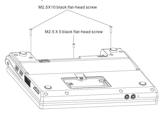
Figure 4-4 Removing the keyboard cover and keyboard
